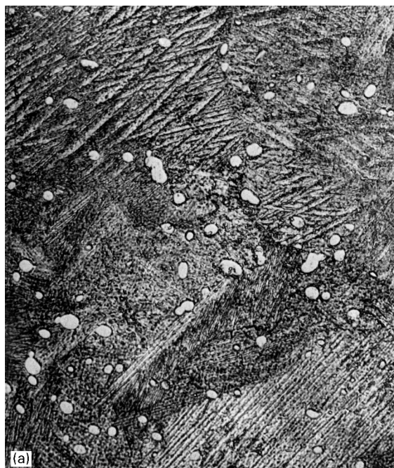
Figure 1 Optical micrographs of the CANTiM alloy photographed at RT: (a) directly-quenched; (b) DQ followed by heating at 573 K for 2 h; (c) DQ followed by heating at 623 K for 2 h.
